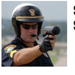
The performance and range of a vehicle-mounted radar in a versatile, hand-held lightweight package. The Stalker II includes direction-sensing and moving mode technology and is available in either moving / stationary or stationary-only versions.
