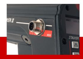
The Stalker II MDR can be purchased with an optional rear antenna port. With this feature, a second, rear-facing antenna can be connected to the Stalker II MDR to yield the performance of a two-antenna dash-mounted unit either in a patrol vehicle or on a motorcycle.
